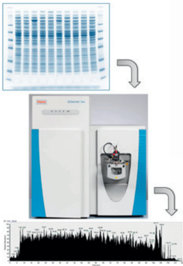
Figure 1. Overview of mass spectrometry sample workflow. Proteins are visualised in a Coomassie Brilliant Blue-stained SDS polyacrylamide gel and subsequently digested to peptides for measurement using a high-resolution mass spectrometer platform (Q Exactive Plus). The chromatogram depicts the usual analysis of a highly complex protein sample.
